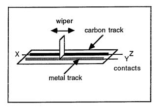
The operating shaft is joined to a metal wiper. This makes contact with the carbon track resistance element X-Z and also to a metal track running alongside which provides the wiper contact Y.
