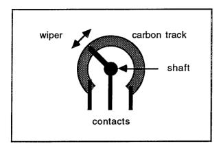
The resistance element is a 270° substrate on which a film of graphite is deposited. A fingered metal wiper moves around the track when the shaft is turned. If the wiper and one end contact are used the device is strictly-speaking called a **variable resistor**. If a voltage is applied across the ends and 'tapped off' by the wiper the device is properly termed a **potentiometer**.
