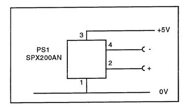
No external components are required. The output voltage will show a permanent differential which varies with barometric pressure and altitude.
