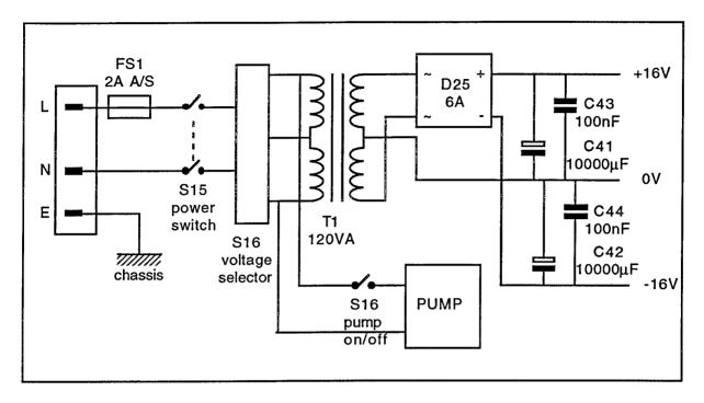
For low induced and radiated noise the 1750 uses linear-mode power supplies.
