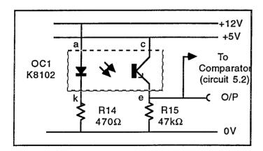
The infra-red L.E.D. has a larger **forward voltage drop** than a silicon diode (1.7V instead of 0.6V) The operating current is set to about 21mA by R14. The phototransistor collector current rises when the beam is admitted and the voltage across R15 rises. A series of positive pulses is generated when the slotted disk is rotated. A comparator monitors the output voltage and lights an indicator L.E.D. This circuit will be found in section 5.2.
