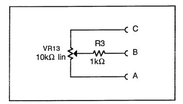
VR13 is a  $10k\Omega$  carbon-track slide potentiometer with a travel of 55mm. approx. The track is protected by R3.
