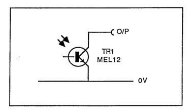
TR1 is a high-gain phototransistor in which the collector current is proportional to the incident light intensity as in the following formula:
