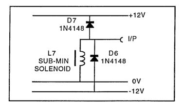
Diodes D6 and D7 clamp the back E.M.F. when power is removed.
