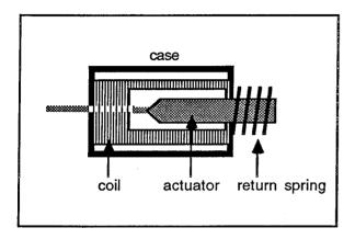
The solenoid takes many different forms. The unit used on the 1750 is a miniature pull-in type. The actuator is a soft iron core which moves inside a high-inductance coil. When the coil is energized the core becomes magnetized in the opposite sense and this causes it to be attracted into the solenoid. When power is removed the core is released by a return spring. A pillar limits the travel on the 1750.
