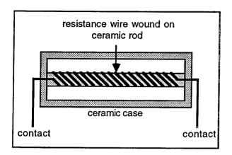
The heater employed by the 1750 is a  $47\Omega$  wirewound resistor. Its construction is identical to many industrial heating elements; it consists of a ceramic rod on which is wound a coil of resistance wire made from a poorly-conducting alloy such as Nichrome or Constantan. The assembly is sealed inside a ceramic case. On the 1750 the heater resistor is mounted inside a clear plastic cover with some temperature sensors.
