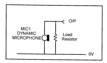
The microphone used on the 1750 has a nominal coil impedance between  $200 - 600\Omega$  and it is important to match this correctly to meet the frequency response specification. Matching is performed by a load resistor. The AC amplifier on maximum gain will be required to obtain a useful signal. Owing to its proximity to the power transformer a certain amount of interference at power line frequency (or harmonics of it) will be induced.
