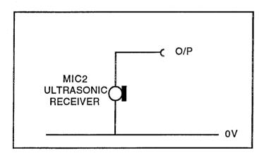
The ultrasonic receiver is mounted in close proximity to the ultrasonic transmitter on the PCB and this results in direct pickup of signals through the board. When an object moves towards the pair the reflected signal is Doppler-shifted so that its frequency changes slightly. The result is a low-frequency modulation of the received signal which can be filtered out and used to detect movement. The receiver has a high output impedance.
