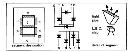
A seven-segment display uses an array of light-emitting diodes to produce the numerals 0-9 and other characters. The standard segment lettering is shown on the left and the corresponding pattern of diodes in the center. Note how all the anodes are joined; this is a **common-anode** display. The visible segments are the ends of translucent plastic light-pipes which funnel up the light from the L.E.D. chips in the base of the display.
