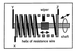
When the shaft is turned a wiper spirals along a track wound helically with resistance wire. X and Z are the track contacts and Y is the wiper contact.
