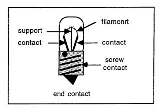
The lamp uses a very fine tungsten filament supported in a mixture of nitrogen and argon gas under low pressure in a glass bulb. The resistance of the filament rises dramatically with increasing temperature and therefore the power dissipation tends to be self-limiting.
