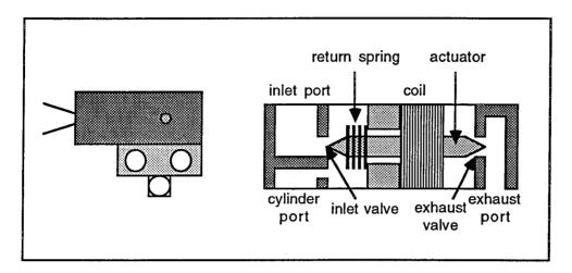
A much-simplified diagram of the air valve is shown above. An actuator operates one of two valves. With no current in the coil the actuator is forced against the inlet valve by a spring. Air can now flow back through the cylinder port and leave via the open exhaust valve and port. If the coil is now energized the actuator is pulled to the right, closing the exhaust port and opening the inlet port. Air can now enter via the inlet port and proceed to the cylinder port.
