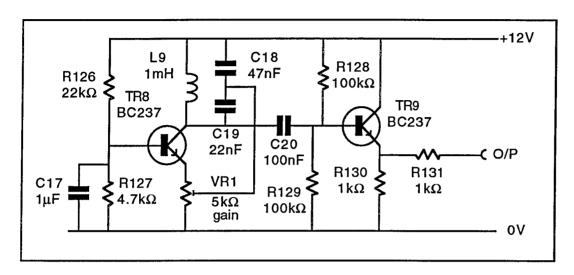
This circuit generates a low-distortion 40kHz sine-wave for many of the A.C.-driven transducers. TR1 is wired as a common-base Colpitts oscillator with base bias set by R126 and R127 and decoupled by C17. The operating frequency **fosc** is set by L9 and the effective series capacitance of C18 and C19 which is 15nF:
