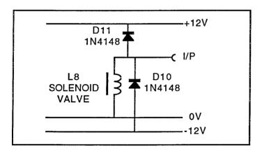
L8 is a 12V solenoid valve. Back E.M.F. spikes are clamped by D10 and D11.
