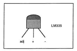
The LM335 temperature sensor is a three-terminal silicon integrated circuit in a plastic TO-92 transistor package. Despite its apparent simplicity it actually contains 16 transistors,9 resistors and 2 capacitors.
