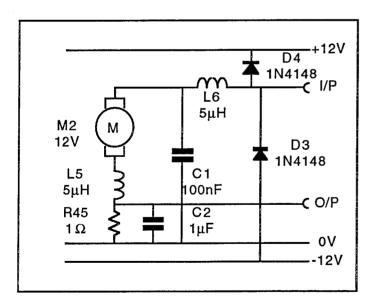
The motor current passes through R44 and develops a voltage across it which is proportional to the torque loading. C2 provides a small amount of noise filtering.L5 ,L6 and C1 reduce radiated R.F. noise and D3 and D4 clamp commutating spikes The voltage across R45 is accessible via the **O/P** socket.
