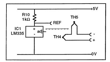
Type K thermocouples are made from chromel and alumel alloy wires. The temperature coefficient of a type K thermocouple is fairly linear in the 0-100°C range at 40.28µV/°C. Due to the very small voltage the use of the instrumentation amplifier followed by several high-gain amplifier stages is recommended. A gain of 248 will provide 10mV/°C
