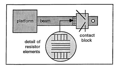
The 1750 strain gauge is a metal beam with a contact block at one end. It has a thin section over which is electro-deposited a network of resistors. Some of these are formed along the axis of the beam and become elongated when it is stressed, thereby increasing in resistance. Others are deposited perpendicular to the beam and provide a reference. The elements are connected in a **bridge** circuit as shown below. Temperature effects are minimized since all the elements are in thermal contact.
