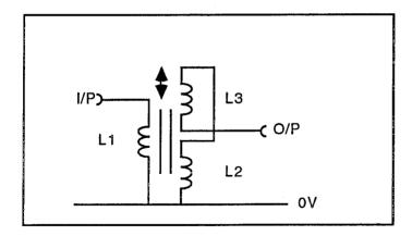
On the 1750 a knurled knob operates a screw which moves the plunger in and out.L1 is the **transmit** coil and L2 and L3 are the **receive** coils.The input should be driven by the 40kHz oscillator. The output should be boosted by the A.C. amplifier and then cleaned up with the 40kHz filter.
