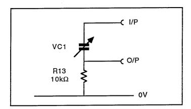
The input should be driven by the 40kHz oscillator and the output boosted by the A.C. amplifier.
