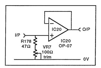
This circuit is basically just a buffered resistor. The input current I develops a voltage IR across R178 and VR7. The voltage is buffered by IC20.
