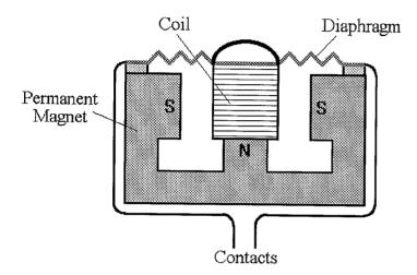
The dynamic microphone operates on the principle that a magnet moved within a coil generates a voltage. In this case the magnet is fixed and the coil is the moving part. The coil is attached to a thin diaphragm which moves in response to sound vibrations in the air. The resulting alternating voltage is supplied to the contacts via very fine wires running along the diaphragm.
