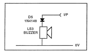
LS3 is a 12V buzzer. Diode D5 is included to protect against reverse voltages.
