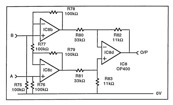
This is one of the standard configurations for an instrumentation amplifier. It is basically a differential amplifier but it scores over circuit 15.5 on several counts; it presents the same impedance on both inputs and the common-mode gain is typically three times lower.
