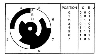
The Gray code is preferred to straight binary for encoded disks because only one bit ever changes at a time, thereby reducing the error that can occur at a segment boundary. The disk used on the 1750 is shown above; black areas produce a low-voltage output from the associated reflective opto sensor while white areas reflect infra-red and produce a high voltage.
