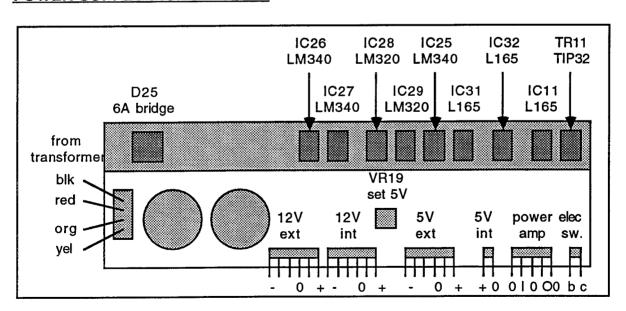
The diagram above shows the external connections and identifies voltage regulators and integrated circuits.
