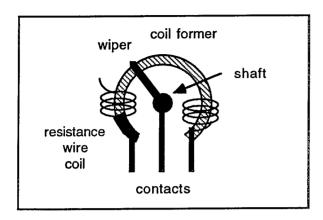
The track consists of a closely-wound coil of resistance wire over which a fingered metal wiper travels when the shaft is turned. The resolution is limited to the resistance of one turn of the coil and is therefore much lower than that of a carbon-track device. This is offset by improvements in other parameters such as stability, temperature coefficient and powerhandling.
