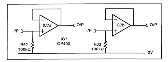
IC7a and IC7b are wired as unity-gain buffers with the outputs connected to the inverting inputs. The circuit performs the task of changing an input signal from high to low impedance while keeping all its other characteristics. The very high input impedance is reduced to  $100k\Omega$  by R62 and R63.
