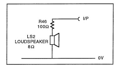
LS2 is an  $8\Omega$ , 200mW loudspeaker with the maximum power dissipation limited to 98mW by R46.
