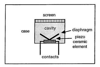
The ultrasonic transmitter contains a piezo-electric element similar to that in the receiver described previously. However, the transmitting device has a lower impedance to permit greater output power for a given input voltage (the devices will in fact work in reverse, but not very well!). Please refer to **section 7.7,Ultrasonic receiver.**
