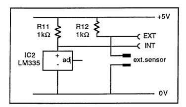
This LM335 provides a linear output of +10mV/°C and the output voltage directly represents the temperature in Kelvin e.g. at 20°C (293K) it will be 2.93V. The chip has an adjustment pin for trimming this voltage but it is not used in this application. A two-pin socket is provided for the connection of an external LM335 probe.
