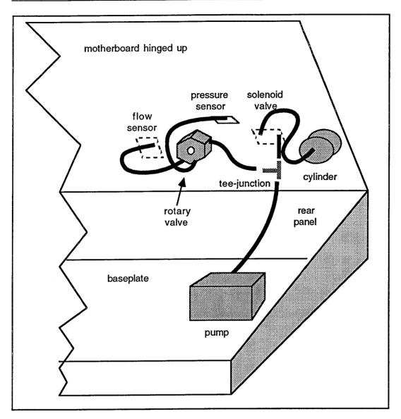
The diagram above shows the 'plumbing' of the 1750. Thick-walled plastic pipe of 6mm outside diameter and 3mm bore is used throughout.
