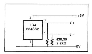
The 634SS2 provides two outputs. The voltage on pin 3 rises when a south pole is brought close while pin 2 falls. The reverse is true for a north pole. R38 and R39 match the  $2k\Omega$  output impedance.
