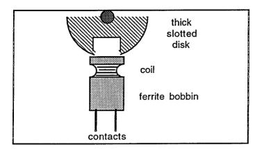
In its simplest form an inductive proximity detector consists of a coil whose inductance changes when a metallic object is brought close. The 1750 employs a 1mH radio-frequency choke coil wound on an open ferrite bobbin. A thick slotted aluminium disk on the drive shaft rotates above the sensor. Commercial inductive sensors use more complex coil arrangements and often include the necessary circuitry within the unit.
