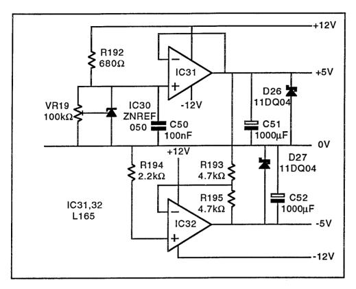
This circuit uses a precision voltage reference and power operational amplifiers to provide an accurate ±5V supply. IC31 acts as a buffer for the voltage reference chip IC30. This device receives its operating current via R192 and voltage trimming is provided by VR19. C50 removes noise. The output of IC31 is decoupled by C51 while D26 prevents negative excursions.
