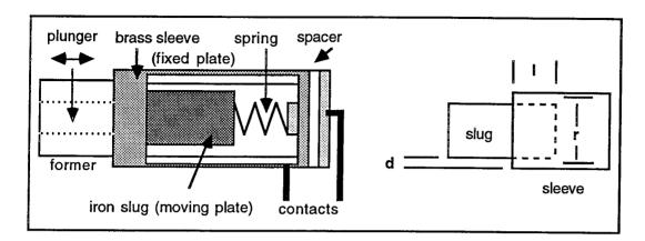
This transducer shares the coil former and plunger with the L.V.D.T. The end of the former is shrouded by a brass sleeve which forms the **fixed plate** of the capacitor. The end of the plunger is joined to an iron slug which moves within the sleeve while insulated from it by the former. The slug is the **moving plate** and electrical contact is made by a spring and endplate. The spring also serves to keep the plunger in tension against its operating screw.
