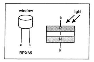
One of the problems with P-N junction photodevices is the electric field which forms across the junction. This manifests itself as a capacitance of typically 100pF which limits the rise and fall time of the photocurrent. To minimize this effect a third layer of **intrinsic** or very lightly-doped silicon can be incorporated. This separates the charged regions and greatly reduces the capacitance to typically 15pF.
