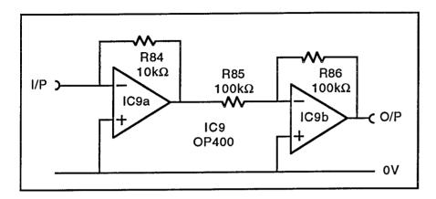
This circuit, which is intended primarily for use with the P.I.N. photodiode, is strictly-speaking a current-to-voltage converter. If a current  $I_{IN}$  is fed into the input the output of IC9a will be  $-I_{IN}$  x R84. This is inverted by IC9b to provide a final output:
