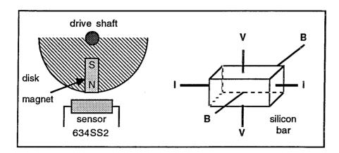
Integrated circuits are available which sense the **presence** or **strength** of magnetic fields and these are known respectively as **Hall effect switches** or **linear Hall effect sensors**. The 1750 employs one of the latter (634SS2) to detect when a small bar magnet is above the chip. This magnet is buried in a thick aluminium disk on the drive shaft.
