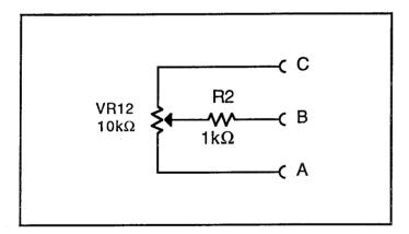
VR12 lis a  $10k\Omega$  wirewound-track potentiometer with nominal 270° rotation.R2 protects the track from excessive dissipation and limits the minimum resistance to  $1k\Omega$ .
