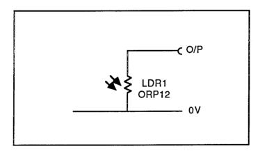
The resistance of the ORP12 drops dramatically as the incident light increases. The device requires a suitable load resistor to provide a voltage output which then falls with increasing illumination.
