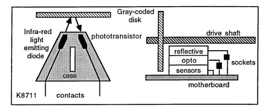
The reflective opto sensor is another device employing an infrared L.E.D. and phototransistor. The components are arranged so that the beam is returned if a reflective surface is placed at the correct distance. For the K8711 this is about 4mm. The 1750 employs three devices mounted in a sandwich with the top pair socketed. The reflective surface is a Gray-coded adhesive overlay on an aluminium disk which revolves with the drive shaft
