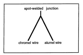
Thermocouples consist of junctions between dissimilar metals. A small but predictable voltage is generated when the junction is heated. To eliminate dissimilar junctions at the soldered ends, two junctions are placed in series. This also gives the opportunity to monitor the absolute temperature of one of the junctions and on the 1750 this is accomplished with a LM335 Kelvin temperature sensor mounted in an aluminium block with one of the the thermocouples.
