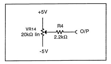
VR14 is a precision  $20k\Omega$  potentiometer designed for use in servo mechanisms. The track is connected permanently between -5V and +5V. The maximum permissible wiper current is 10mA. With a worst-case applied voltage of 17V the  $2.2k\Omega$  series resistor R4 limits the current to 7.7mA.
