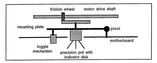
A precision potentiometer is mounted on a moveable plate. This plate is fixed to a sprung toggle mechanism which allows the potentiometer to be operated by the drive shaft via an aluminum disk and rubber friction ring.. The plate is pressed down once to engage the mechanism and again to release. The shaft reduction ratio of this arrangement is 4:1. The potentiometer itself is similar in construction to the carbon pot but it has a 360° conductive plastic track and precision bearings.
