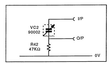
The sensor forms a potential divider with R42. When an alternating voltage is applied to the input an output voltage of the following form is obtained:
