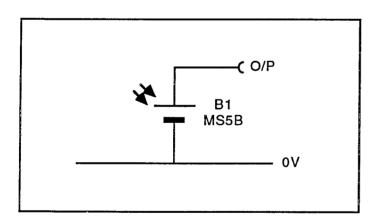
The MS5B has an active area of about 5mm X 13mm. The main parameters of interest are the open-circuit voltage  $V_0$  and short-circuit current  $I_s$ . The open-circuit voltage initially rises logarithmically with increasing light towards a limit of 0.6V. The short-circuit current rises linearly under the same conditions and is also proportional to surface area.
