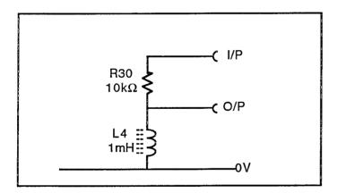
The coil L4 forms a potential divider with R30. If an alternating voltage is applied to the input there will be an output voltage given by the following formula:
