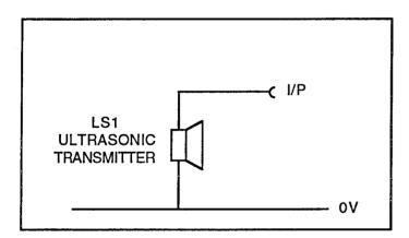
The device should be driven directly by the 40kHz oscillator.
