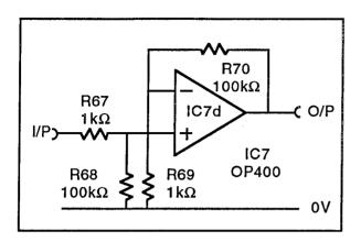
IC7d is wired in the configuration of a non-inverting amplifier. If R67 were omitted the gain would be 1 + R70 / R69, i.e. 101. However, R67 and R68 provide an attenuation of R68 / (R68+R69), i.e. 100/101. The total gain is therefore the product of these which is 100.
