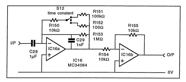
This circuit provides an output which represents the rate of change of the input signal . This is multiplied by a time constant **RC** that is determined by the input capacitor C28 and the feedback resistor combination selected by S12. The circuit is prone to noise pickup and this is reduced by C29. The signal is inverted by IC16b and associated components. The final output is of this form :
