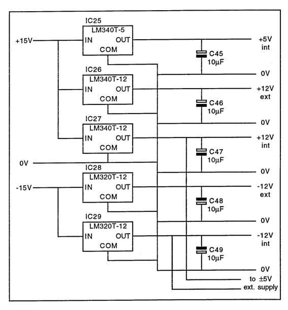
These power rails all make use of three-terminal linear voltage regulators. The devices are mounted on a heatsink attached to the power supply PCB. C45-C49 are required for stability.
