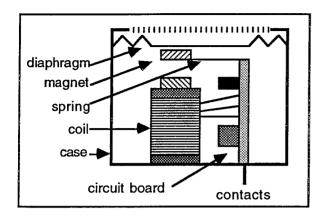
There are many different kinds of buzzer. The device used by the 1750 employs a small transistorized oscillator to generate an alternating magnetic field in a coil. This coil has an iron pole-piece which attracts and repels a small permanent magnet attached to a spring. The magnet vibrates against a diaphragm and creates a very loud noise.
