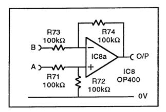
IC8a is wired in the standard differential amplifier configuration. If the voltage on **A** is held constant while **B** is varied the gain will be - (R74 / R73), i.e. -1. If **B** is now held constant and **A** varied the gain will be:
