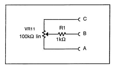
VR11 is a  $100k\Omega$  carbon-track potentiometer. The track is protected by R1 which limits the worst-case power dissipation to 288mW. When used as a variable resistor rather than a potentiometer the minimum resistance will be  $1k\Omega$  accordingly.
