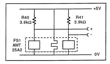
Both sensors have  $3.9k\Omega$  load resistors. The heated sensor drives the (-) output. Since it has a positive temperature coefficient the output voltage will fall when air flows past.
