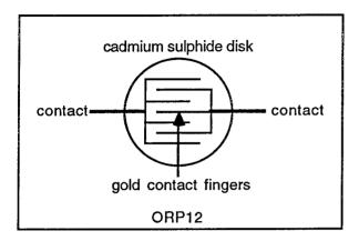
Photoconductive cells are made from cadmium sulphide doped with silver, antimony or indium chemically deposited on a substrate with interleaved gold contact fingers formed on top. Light falling on the sensitive area breaks chemical bonds. The resulting electrons and holes become available to increase the conductivity. These bonds are slow to re-form when light is removed and the response time is sluggish.
