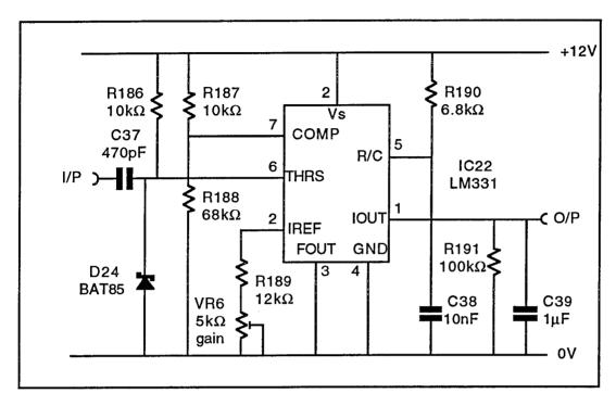
In this application a pulse train applied to the input is differentiated by C37. Each negative-going edge causes the monostable multivibrator in the 331 to fire and a packet of charge is dumped on C39 thereby raising its voltage . The voltage falls until the next charge pulse is received and the average level is proportional to the input pulse frequency. With  $1\mu F$  for C39 the response time is slow but the ripple is less than 10mV.
