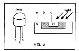
The phototransistor has three layers of silicon containing tiny amounts of impurities. These layers are termed **emitter,base** and **collector**. When a positive voltage is applied between collector and emitter a tiny **reverse saturation current** flows. This current is due to electrons and holes created by warmth. The geometry of a phototransistor allows light to shine on the collector-base junction and this creates additional current carriers. This current is amplified by transistor action.
