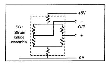
The strain gauge is connected across the +5V supply. When the beam is loaded the (+) output voltage rises and the (-) output falls. Damage due to over-bending is prevented by a restraining bridge. The output is typically a few microvolts and the use of the instrumentation amplifier followed by high-gain stages is recommended.
