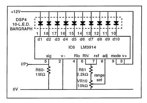
IC6 (LM3914) is a dedicated bargraph driver chip. It compares the input voltage with ten internal references and turns on the corresponding number of L.E.Ds. R60 grounds the input with no signal applied. R61 sets the display current and VR10 sets the voltage increment between L.E.Ds.
