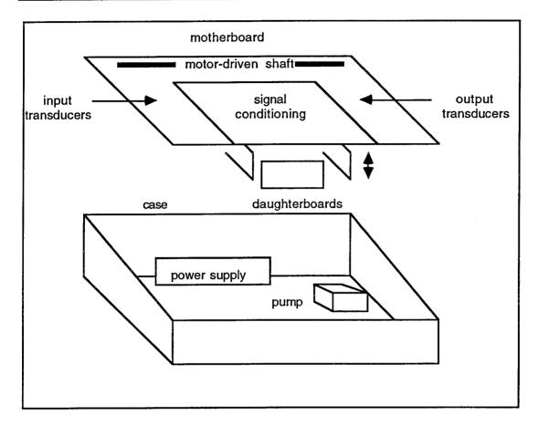
The DIGIAC 1750 is a self-contained trainer designed to introduce students to many of the techniques involved when working with transducers. The unit allows the investigation of the properties of various input and output devices and of the various methods of signal-conditioning required.
