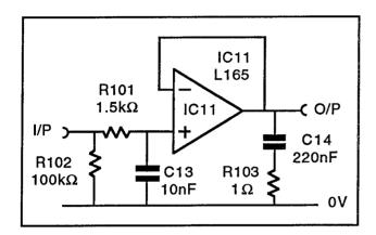
IC11 is a power operational amplifier in a five-pin TO-220 plastic case. It requires a heatsink and for this reason the circuit is included on the power supply P.C.B. with connection made to the motherboard by a five-way cable. IC11 is configured as a unity-gain buffer. C14 and R103 are a **Zobel network** and are essential for stability. R101 and C13 form a filter with a 10kHz break to attenuate 40kHz signals.
