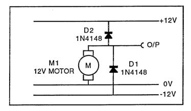
Diodes D1 and D2 clamp commutating spikes to  $\pm 12.7$ V. The output may require low-pass filtering to remove noise.
