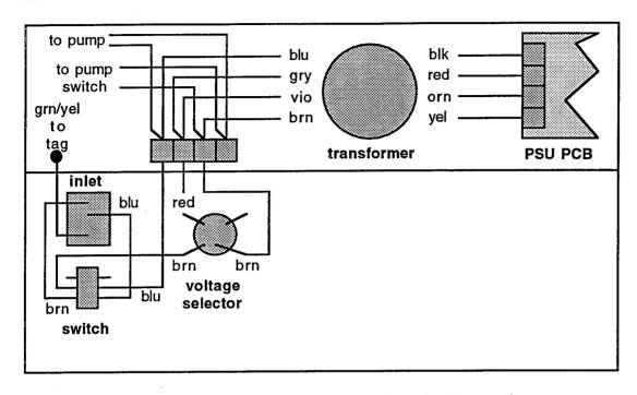
The wiring layout for the rear panel and baseplate is shown above.
