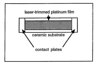
The RTD consists of a thin film of platinum deposited on a ceramic substrate with gold contact-plates on each end. The film is laser-trimmed to precisely  $100\Omega$  at  $0^{\circ}$ C.
