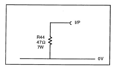
With the maximum applied voltage of 12V the output power will be 3W. The temperature rises to about 40°C above ambient, taking about 5 minutes before levelling out.
