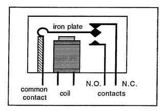
A miniature changeover relay is used on the 1750. It has a common terminal which is attached to a springy contact strip. The **common** contact is on the end of this strip and is held against the **normally closed (N.C.)** contact by the spring. When power is applied to the coil it attracts the iron plate and causes the common contact to engage the **normally open (N.O.)** contact. The contacts 'bounce' for a short period each time they **make** and **break**.
