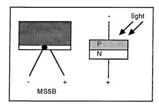
The photovoltaic cell is a two-layer silicon device. It generates a voltage by electron/hole pair production when the junction is exposed to light. These diffuse across the junction to set up a voltage. A current will flow if a resistance is placed across the terminals. Devices optimized for energy production are often called **solar cells**.
