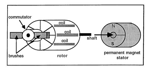
The D.C. motor employed by the 1750 is identical to the unit which was described in its other guise as a tachogenerator. In this application current is supplied to the coils via the brushes and commutator and this causes forces to be exerted on the rotor which make it spin. Please refer to **section 5.5,Tachogenerator** for a fuller description of the component parts. Note the very high efficiency shown in the table of characteristics.
