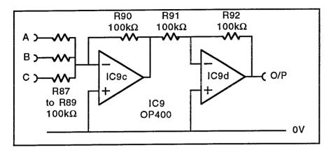
IC9c is a conventional inverting summer providing an output of -  $(V_A + V_B + V_C)$ . This is inverted by IC9d so that :
