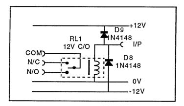
Back E.M.F. spikes when power is removed are clamped by D8 and D9.
