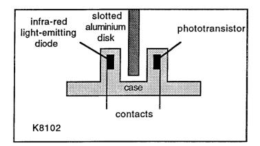
This device consists of a gallium arsenide infra-red L.E.D. and silicon phototransistor mounted in a special plastic case which is transparent to light of this wavelength. The elements are separated by a slot which allows the beam to be broken when an infrared-opaque object is inserted. On the 1750 the obstruction is provided by a slotted aluminium disk on the motor drive shaft.
