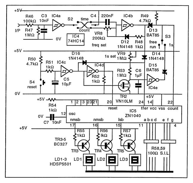
This unit is not a transducer in the accepted sense, although it does use L.E.D. seven-segment displays. However, the counting of events and the measurement of time are often important considerations when working with transducers. This unit provides three basic functions; counting up to 999 events, counting number of events in one second and timing an event in multiples of 10ms. A single active-high input is provided and count/time are shown on three seven-segment L.E.D. displays.
