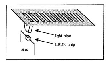
This consists of ten gallium arsenide/phosphide light-emitting diodes in a 20-pin I.C. package. The light from each chip is collected by a light-pipe and emitted as a bar.
