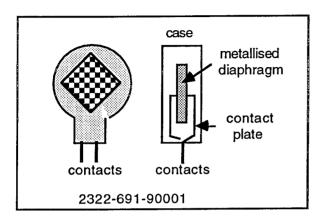
This device comprises a very thin diaphragm constructed from a special dielectric material whose properties change with atmospheric humidity. The diaphragm is metallized on both sides to form a capacitor which changes in value with the dampness of its surroundings. The element is housed in a slotted plastic case.
