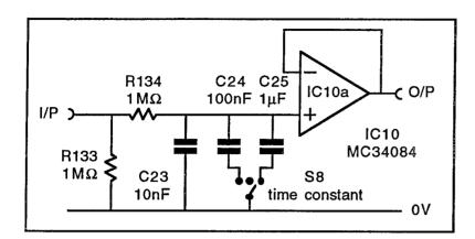
Circuit 16.3 is a simple buffered single-pole low-pass filter. The time constant is determined by the product  $\mathbf{CR}$  where  $\mathbf{C}$  is C23 either on its own or in parallel with C24 or C25 dependant on switch position.  $\mathbf{R}$  is R134 (1M $\Omega$ ) giving approximate time constants of 10ms, 100ms and 1s. These could also be expressed as break frequencies given by :
