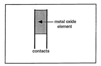
The NTC thermistor is a two-terminal semiconductor device with an element made from sintered oxides of metals such as nickel, manganese and cobalt.
