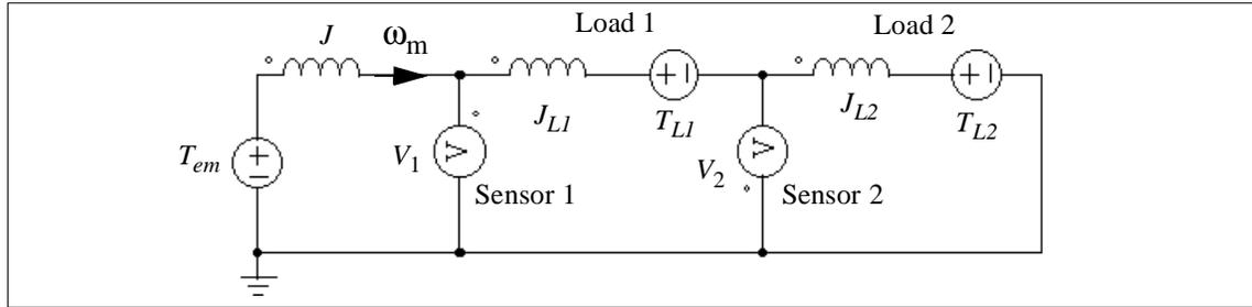
The current in the circuit represents the mechanical speed  $\omega_m$ . The voltage probe  $V_1$ , which measures the node-to-ground voltage at the machine shaft output, represents the reading of the torque sensor No. 1. Similarly, the probe  $V_2$  represents the reading of the torque sensor No. 2. Note that the probe  $V_2$  is inverted (from the ground to the node) since Sensor 2 is against the reference direction of the mechanical system.
