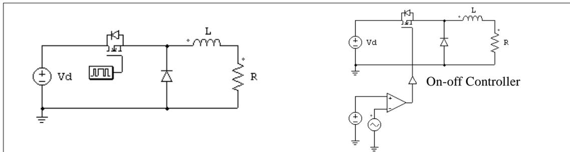
The circuit on the right uses an on-off switch controller (see Section 4.7.1). The gating signal is determined by the comparator output.
