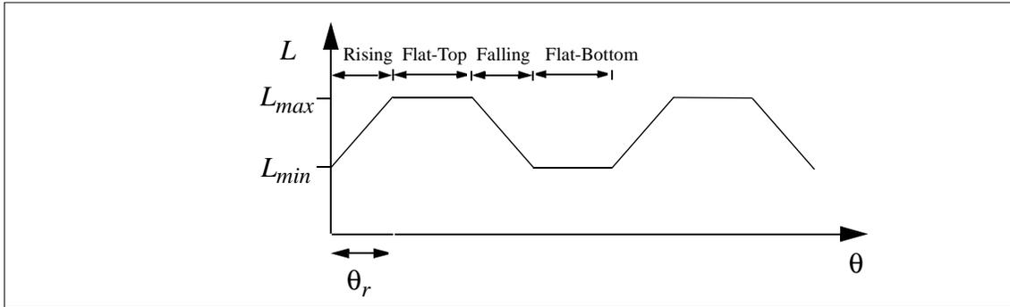
The rotor angle is defined such that, when the stator and the rotor teeth are completely out of alignment,  $\theta = 0$ . The value of the inductance can be in either rising stage, flat-top stage, falling stage, or flat-bottom stage.
