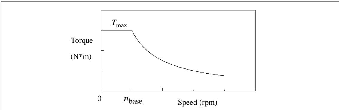
When the mechanical speed is less than the base speed  $n_{\text{base}}$ , the load torque is:
