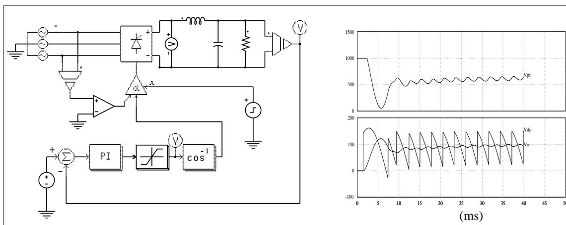
The rectifier is controlled through an alpha controller. The synchronization of the controller is provided by the zero-crossing of the line voltage  $V_{ac}$ . The alpha value is created through the load voltage feedback loop.
