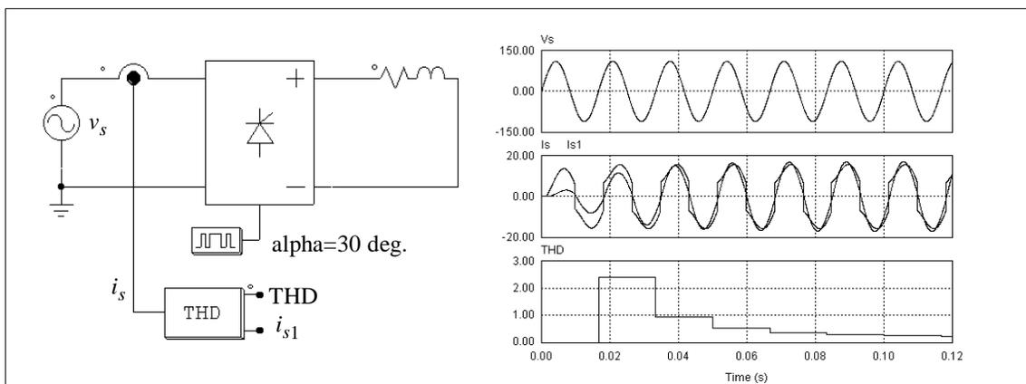
One of the THD block output is the input current fundamental component  $i_{s1}$ . By comparing the phase difference between the input voltage  $v_s$  and the current  $i_{s1}$ , one can calculate the input displacement power factor. This, together with the THD value, can be used to calculate the input power factor.
