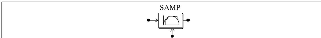
The node at the bottom of the block is for the control signal input.
