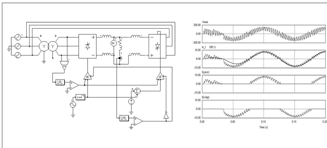
The simulated waveforms of the load voltage, load current (before and after the band-pass filter), and the currents through the positive and negative rectifier bridges are shown below:
