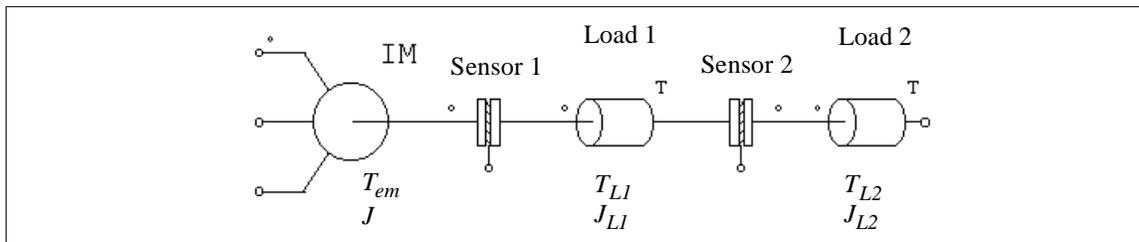
The system consists of one machine, 2 torque sensors, and 2 mechanical loads. The torques and moment of inertia for the machine and the loads are as labelled in the diagram. The reference direction of this mechanical system is from left to right. The equation for this system can be written as:
