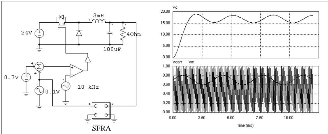
The simulated waveforms of the load voltage, modulation wave and the carrier wave are shown on the right.
