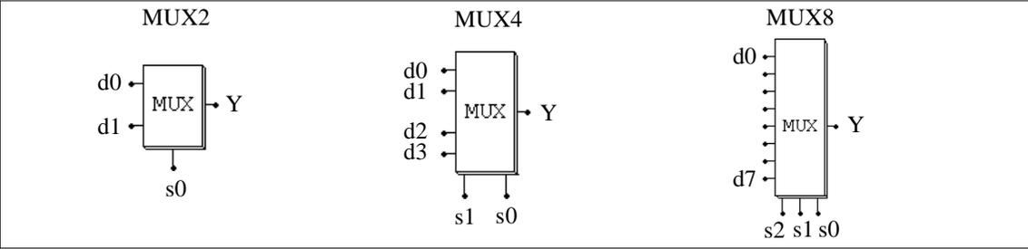
In the images, d0..d7 are the data inputs; and s0..s2 are the control signals. The truth tables of the multiplexers are:
