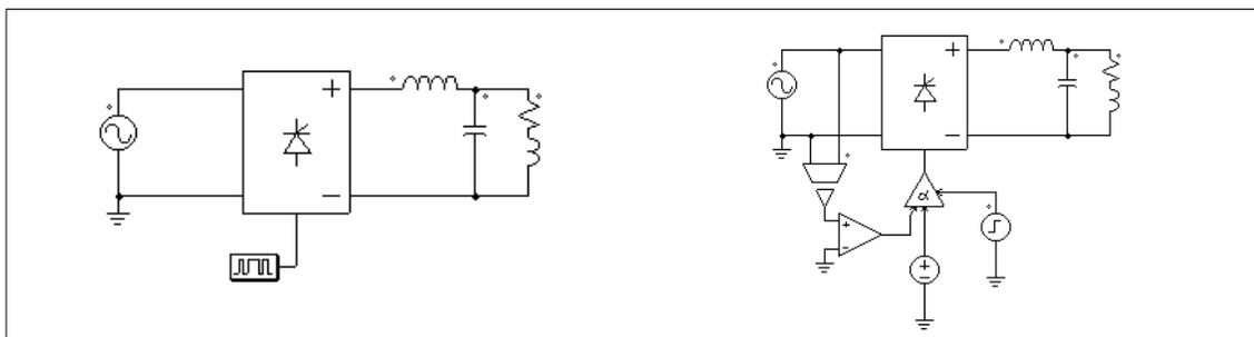
The gatings for the circuit on the left are specified through a gating block, and on the right are controlled through an alpha controller. A major advantage of the alpha controller is that the delay angle alpha of the thyristor bridge, in degree, can be directly controlled.
