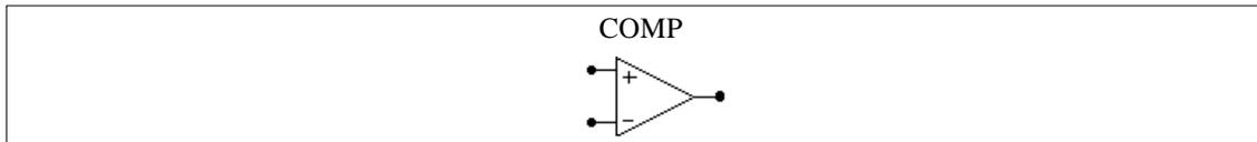
Note that the comparator image is similar to that of the op. amp. For the comparator, the noninverting input is at the upper left and the inverting input is at the lower left. For the op. amp., however, it is the opposite.
