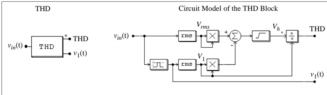
A second-order band-pass filter is used to extract the fundamental component. The center frequency and the passing band of the band-pass filter need to be specified.
