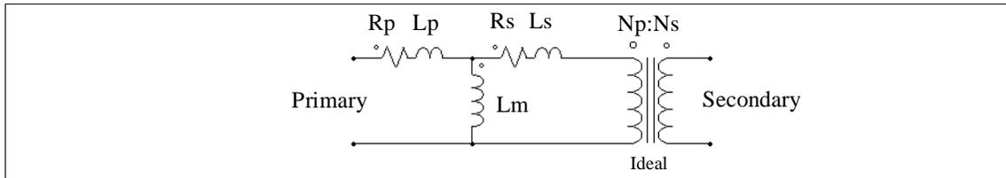
where  $R_p$  and  $R_s$  are the primary/secondary winding resistances;  $L_p$  and  $L_s$  are the primary/secondary winding leakage inductances; and  $L_m$  is the magnetizing inductance. All the values are referred to the primary side.
