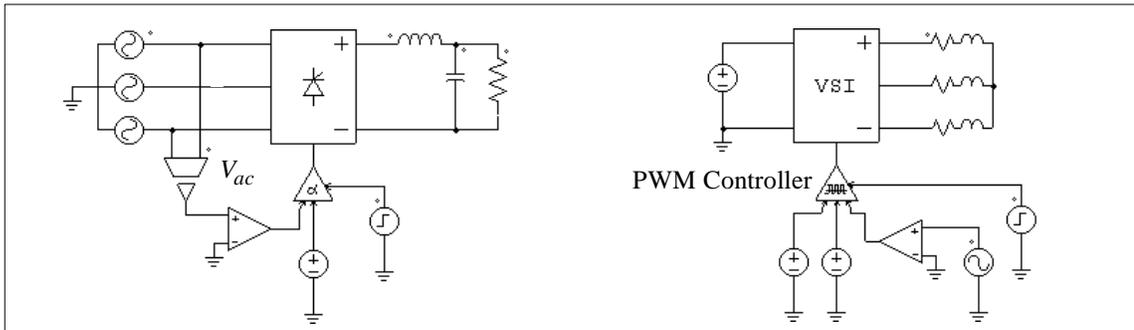
The thyristor circuit on the left uses an alpha controller. For a three-phase circuit, the zero-crossing of the voltage  $V_{ac}$  corresponds to the moment when the delay angle  $\alpha$  is equal to zero. This signal is, therefore, used to provide synchronization to the controller.
