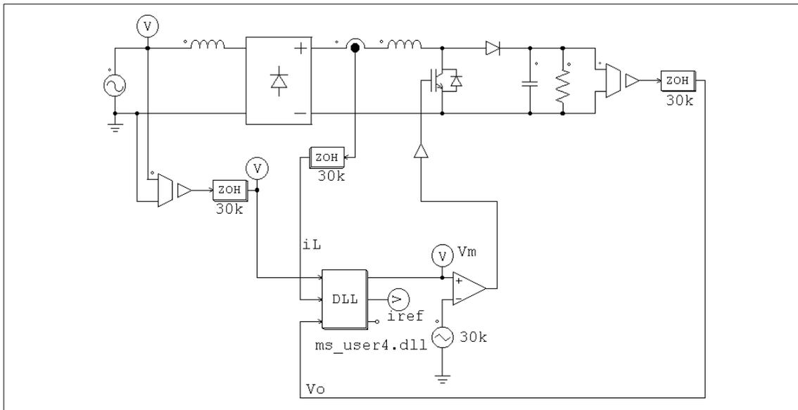
The source code, which is stored in the file “ms\_user4.c”, is shown below. Both the inner current loop and the outer voltage loop use a PI controller. Trapezoidal rule is used to discretize the controllers. Discretization using Backward Euler is also implemented but the codes are commented out.
