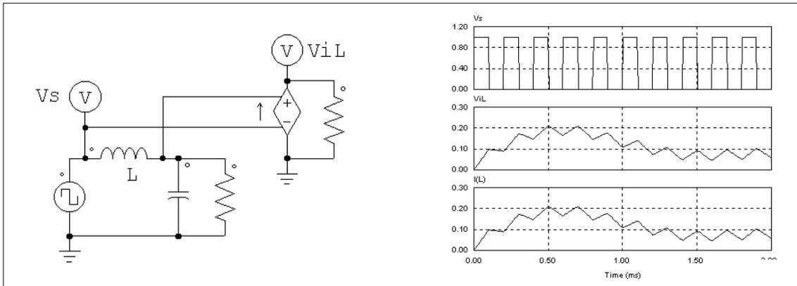
The voltage source is controlled by the branch current  $i_s$ . With a gain of 1, the waveform of the voltage  $v_{i_s}$  is identical to that of  $i_s$ .
