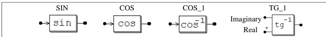
For the arc tangent block, the dotted node is for the real input and the other node is for the imaginary input. The output is the arc tangent of the ratio between the imaginary and the
