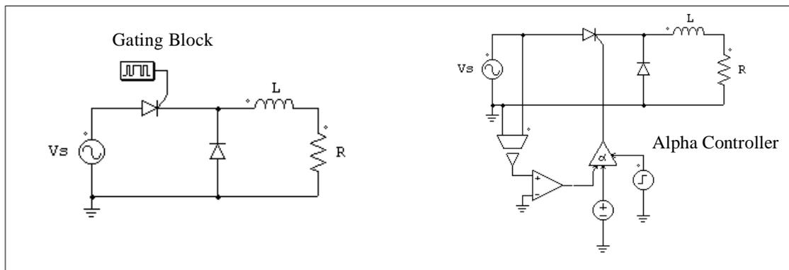
This circuit on the left uses a switching gating block (see Section 2.2.4). The switching gating pattern and the frequency are pre-defined, and will remain unchanged throughout the simulation. The circuit on the right uses an alpha controller (see Section 4.7.2). The delay angle alpha, in degree, is specified through the dc source in the circuit.
