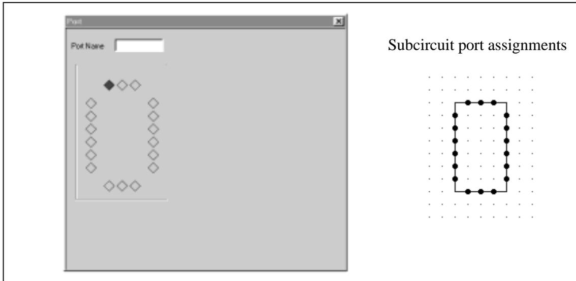
The diamonds on the four sides represent the connection nodes and the positions of the subcircuit. They correspond to the connection nodes of the subcircuit block on the right. There are no diamonds at the four corners since connections to the corners are not permitted.
