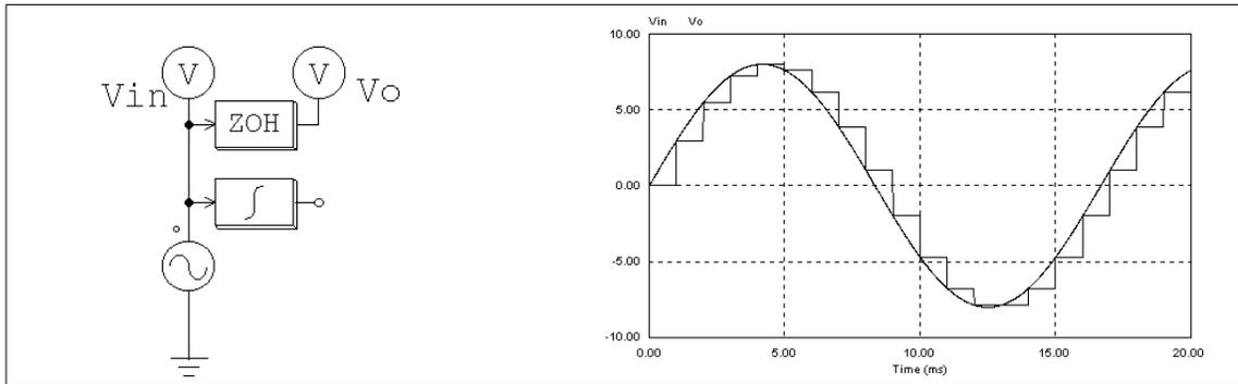
Note that in above circuit, a continuous-domain integrator is also connected to the input sine source. This makes it a mixed continuous-discrete circuit, and a simulation time step selected for the continuous circuit will be used. With this time step, the familiar staircase-like waveform can be observed at the zero-order hold output.
