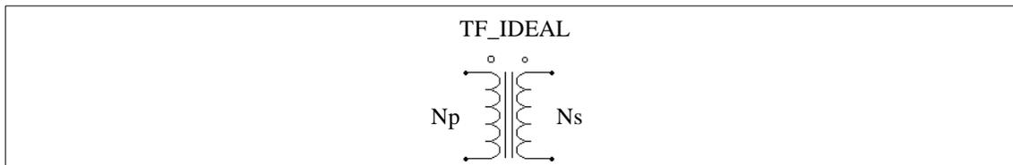
The winding with the larger dot is the primary and the other winding is the secondary.
