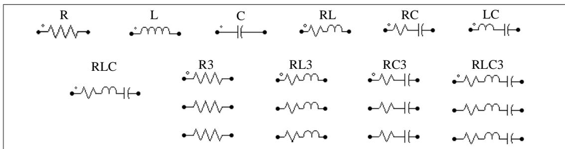
For the three-phase branches, the phase with a dot is Phase A.
